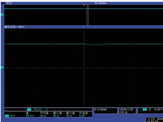
Output dynamic response waveform under 10% ~ 50% load change
