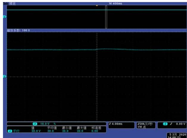
Output dynamic response waveform under 50% ~ 10% load change
