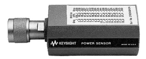
The 8483A diode power sensor measures average power over the frequency range 100 kHz to 2 GHz and power range -30 to +20 dBm (50 dB dynamic range)
