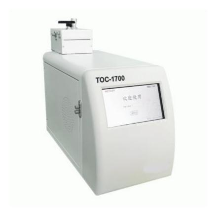
Unlike TOC-2000 and TOC-3000, TOC-1500 and TOC-1700 are equipped with direct conductometric detection method. TOC-1500 is off-line while TOC-1700 integrated on-line sampling while enables easy and quick sample introduction. This series TOC is ideal for application in microelectronics water, purified water, water for injection, cleaning validation and etc. Features
