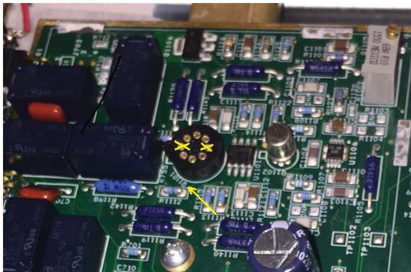
Figure 5.2: The front-end JFET (Q1101) socket, un-installed.
