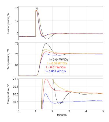
**Derivative**: derivative feedback reduces the heater output whenever the temperature is rising rapidly. In the example below, when the derivative gain *D* is increased from 3 to 6 W·s/°C, the amount of overshoot and oscillation decreases. The temperature rise is also a little slower, but because there is less oscillation the system stabilizes at 70°C sooner.
