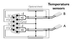
A four-wire connection is used so that the PTC323 measures the resistance of the sensor and not the wires going to the sensor. The +I and -I pins provide a small current and should be connected to the temperature sensor with two wires, preferably a shielded twisted pair. The +V and -V pins measure the voltage produced across the sensor and should be connected to +I and -I as close as possible to the sensor.
