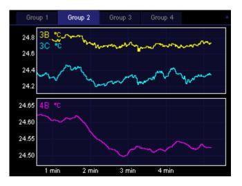
In custom plot mode, the user can manually assign each channel to a graph. Here the thermocouple inputs have been assigned to plot 1 and the RTD input to plot 2.
