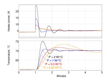
Interestingly, decreasing the proportional gain to 0.5 or  $0.25 \text{ W/}^{\circ}\text{C}$  also results in more overshoot and can even cause oscillations, despite the fact that the heater response is smaller and the temperature rise slower. By reducing the proportional feedback response, we've forced the integral feedback to take more responsibility for raising the heater power — and as the next figure illustrates, the integral feedback has a greater tendency to overshoot and oscillate.
