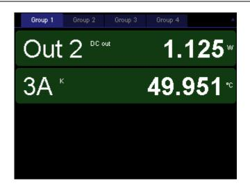
This screen displays the current values of the selected channels as numbers. The more channels that are selected, the smaller the displays are. If enough space is available, an annunciator may appear that indicates whether the sensor or heater is disconnected ("N/A"), over range ("Hi"), under range ("Lo"), if outputs are disabled ("Off"), or if an internal error has occurred ("Err").
