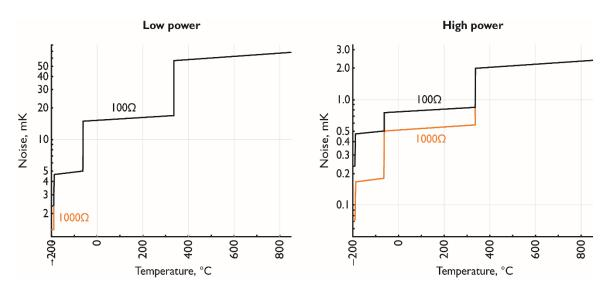
RMS noise levels for  $100 \Omega$  and  $1000 \Omega$  platinum RTD sensors as a function of temperature. At low power, the  $100 \Omega$  and  $1000 \Omega$  sensors have about the same noise level.
