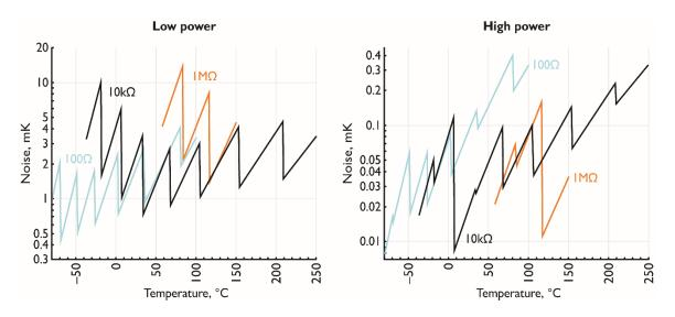
RMS noise levels for  $100 \Omega$ ,  $10 k \Omega$ , and  $1 M \Omega$  (at 25 °C) thermistors as a function of temperature
