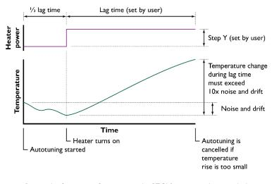
During the first stage of autotuning, the PTC10 compares how much the temperature changes before vs. after turning the heater on. Autotuning is cancelled if the temperature doesn't change 10x more after the heater is turned on.
