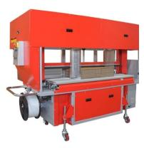
TP-702CQ3-S is an all-electric high-speed corrugated strapper with integrated squaring and backstop functions. It is built on the quality proven Transpak TP-702C corrugated strapper and carries all the innovative features of the TP-702C. Motorized squaring and backstop devices provide precise bundle handling and positioning for forming perfect bundles. It can meet the speed requirement of the fastest Flexo Folder Gluer and Casemaker.
