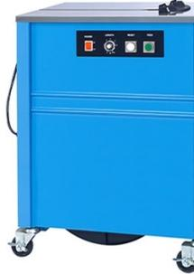
TP-203 is a mini-type semi-auto strapping machine with smoke exhaust system. It is designed specifically for the use in office, bank, post office, book and department store, etc.
