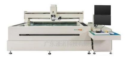
Automatic tool metallographic measuring instrument V2000
