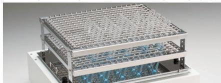
C type: for erlenmeyer flask and test tube
