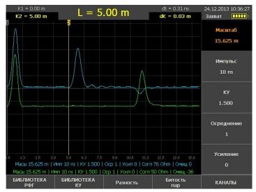
instrument and the overlapping attenuation. In short areas with little attenuation, it is better to use short pulses to provide the best resolution; On long routes with a large attenuation, a longer pulse widths must be set to ensure maximum range;
