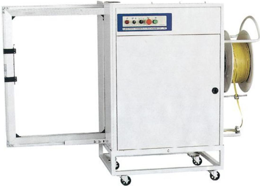
Electrical configuration: "OMRON", "PLC" control, French "TE", and photoelectric switch control.
