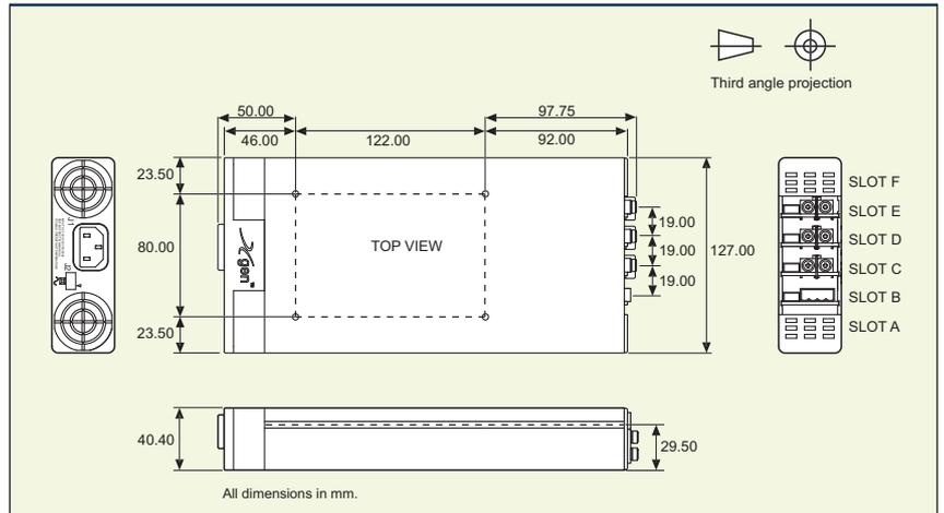
**SPECIFICATION** applies to configured units consisting of *powerMods* plugged into the appropriate *powerPac*
