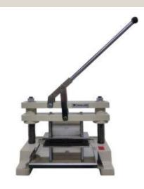
This device is used to extract paper board test specimens for the ring crush test. The operator can easily obtain test specimens by just lowering the lever.
