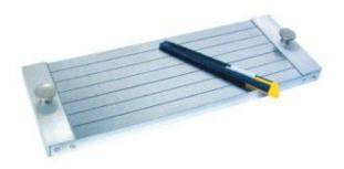
This device enables the operator to exactly extract paper, paper board, and plastic film test specimens for the tensile test. The operator is to cut the test specimen by placing the cutter knife in the grooves of the device.
