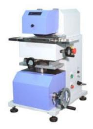
This tester is used to adjust the thickness of vulcanized rubber for test preparation. The thickness of the rubber sample attached to the table is adjusted by moving sample table towards the abrasion wheel.
