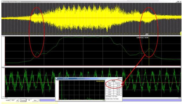
Resonance, at 62.5Hz, appears at both startup and shutdown period
