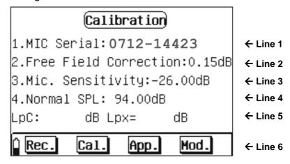
Fig. 35: Initial screen of calibration section
