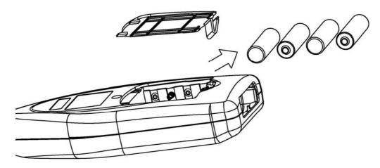
Fig. 55: Replacement of internal batteries
