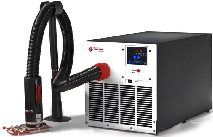
User-programmable temperatures, graphing, and data logging are established through the controller's touch-screen or remote communications. The system provides fast and precise transitions of temperature at the IC, even with variations in device power, and can be used with Temptronic's proven DUT Control technology using an imbedded diode or external thermocouple.
