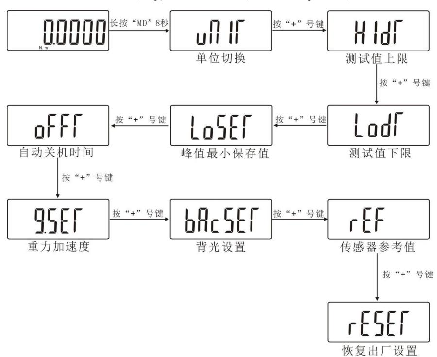
3.1.2 (UNIT) Unit setting: The instrument can switch 3 units, after entering the unit setting interface, press \"+ \"和\"-\" Key to select the unit, as shown below:
