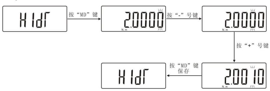
3.1.4 LDD (LODT) Test value lower limit setting: Set the test value lower limit. Below the lower limit is out of range, \"MIN\"display,The lower limit of this instrument defaults to0. If you want to reset the lower limit, under this setting item, use \"+\"with\"-\"Key setting. Press \"MD\"Key to save and return to the setting interface. As shown below:
