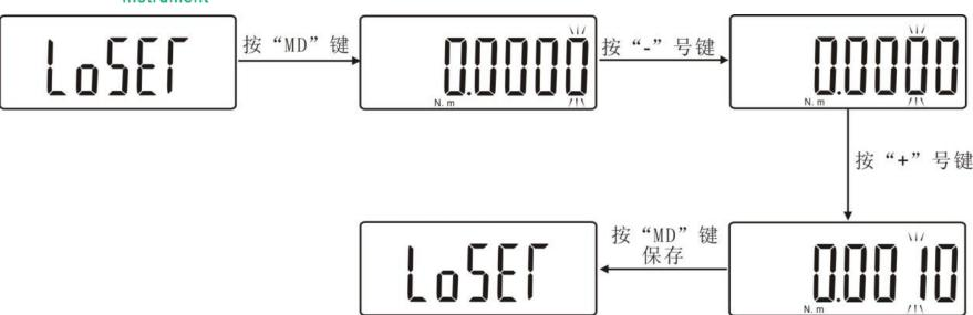
3.1.6 (OFFT) Automatic shutdown time setting:本 Instrument defaultAutomatic shutdown timeFor 10 minutes。Under this setting item, use \"+ \" and \"-\"键 Select, can be set from 0 minutes to 99999Automatic shutdown in minutes, can also be set \"000000 \"Does not automatically shut down. If you do not want to shut down automatically, press \" MD \"to complete the setting after selection and return to the setting interface.As shown below:
