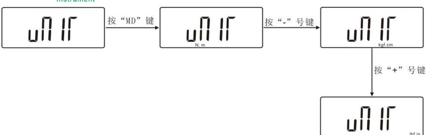
3.1.3 (HIDT) Test value upper limit setting: Set the test value upper limit. Above the upper limit is out of range, \"MAXdisplay\", The default upper limit value of this instrument is full scale. If you want to reset the upper limit, under this setting item, you can use \"+\"with\"-\"Key setting. Press \"MDAfter saving, return to the setting interface. As shown below:
