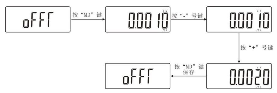
3.1.7 (G.SET) Gravity acceleration setting: the user can set the gravity acceleration value according to the location of the region, This instrument The default is 09.800. Under this setting item, you can use \"+\" and \"-\" keys to set the gravity acceleration setting value. As shown below:
