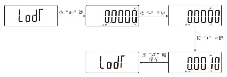
3.1.5 L D D L (LOSET) Minimum saved value of peak value:Minimum peak saved value,The minimum stored value of the peak value of this instrument defaults to0. In peak mode, when the current value is less than this value, the peak value will not be saved. Under this setting item,use\"+\"with\"-\"key 可 set upPeak minimum saved value。As shown below:
