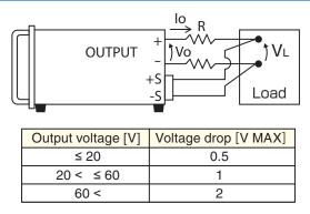
Prevents voltage drop down (Vo-VL) due to resistance (R) or deterioration of stability by contact resistance.
