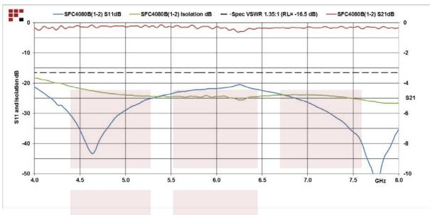
Circulator SMA Female With 17 dB Isolation From 4 GHz to 8 GHz Rated to 10 Watts from Fairview Microwave is in-stock and available to ship same-day. All of our RF/microwave products are available off-the-shelf from our ISO 9001:2008 certified facilities in Allen, Texas. Fairview Microwave is RF on-demand.
