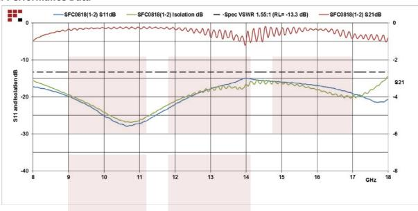
Circulator SMA Female With 13 dB Isolation From 8 GHz to 18 GHz Rated to 10 Watts from Fairview Microwave is in-stock and available to ship same-day. All of our RF/microwave products are available off-the-shelf from our ISO 9001:2008 certified facilities in Allen, Texas. Fairview Microwave is RF on-demand.
