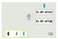
Information on which units are paired to the display unit is displayed. The display unit will only communicate with units that are paired.
