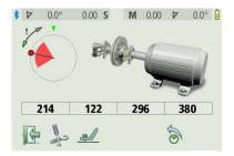
Rotate the shafts to the next position. The shafts must be rotated over a minimum of 45°.
