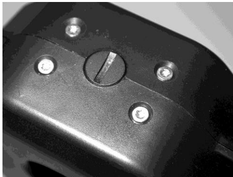
Fig. 11: Internal calibration switch in 'measurement' position.
