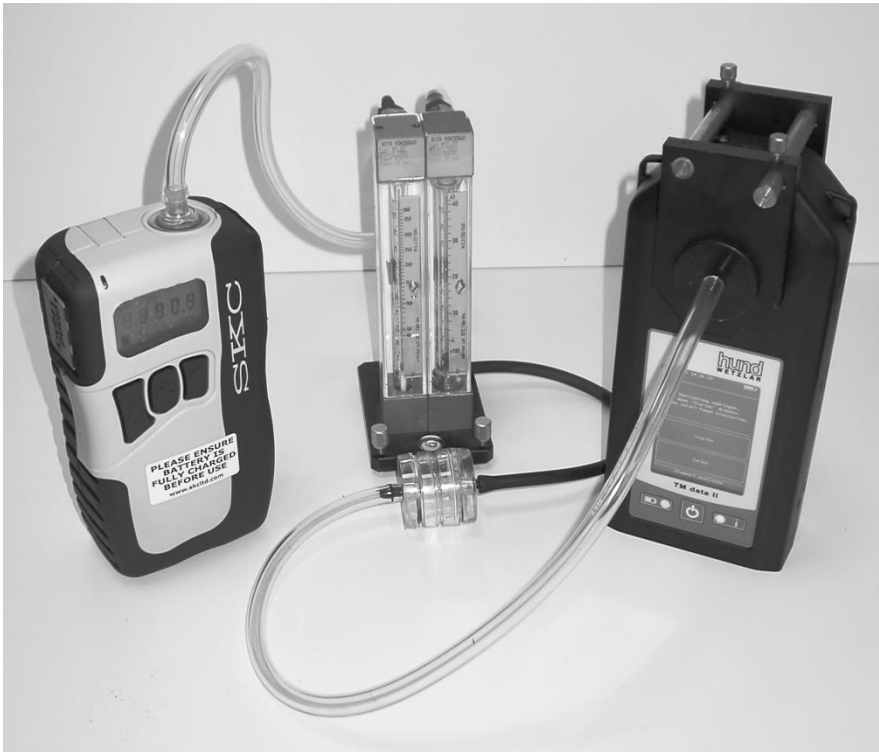
Fig. 12: TM data II calibration set. From left to right: pump, rotameter with total-dust collector (in front of it), TM data II with mounting bracket.
