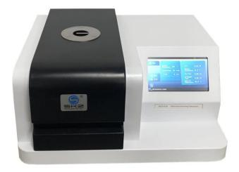
DSC is designed to determine the inner heat transition relating to temperature and heat flow, it is widely used in the field of polymer development, performance testing & quality control. DSC research and development includes the following field: glass transition temperature, melting point, cold crystallization, crystallization, phase transition, oxidation induction time (OIT).
