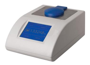
To measure refractive index nD and sugar content (Brix) of transparent and translucent liquid
